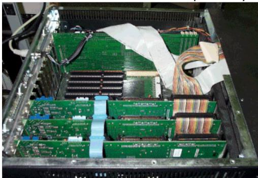
The AV100 card has two built in SCSI controllers, allowing for two separate buses. When connecting AV100 cards and drives, a 50-conductor cable connects everything together.
