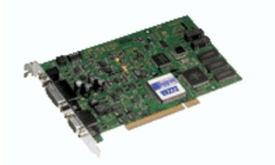
Each card is capable of handling a single record **or** multiple play stereo channels. An analogy can be made with a Record/Play cart machine. Multiple cards can be installed to provide additional stereo channels.
