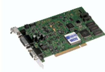
Each card is capable of handling a single record **or** multiple play stereo channels. An analogy can be made with a Record/Play cart machine. Multiple cards can be installed to provide additional stereo channels.
