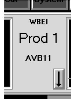
Custom lines are added manually to the AUDIOVAU.INI in either the screen section ([AVRPS], [AVSAT]) or the card section ([AVB11], [PCR41]). You can also define the Custom lines in AVCFG.
