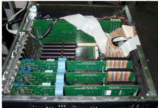
The AV100 card has two built in SCSI controllers, allowing for two separate buses. When connecting AV100 cards and drives, a 50-conductor cable connects everything together.
