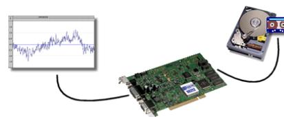
**Sample rate** applies to how many snapshots, or samples, are recorded over a second of audio. The more samples there are per second of audio, the more accurate the recreated waveform can be. A 44.1K sample rate means that 44100 samples are recorded every second.
