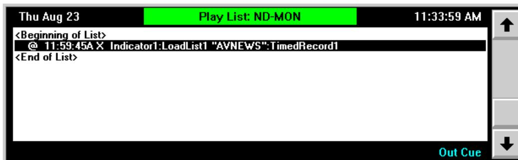
This line says **at 11:59:45A, switch the switcher to the BEI Network, load a cut called AVNEWS into deck 1, and set deck 1 to timed record so the new audio will record over the existing audio.**
