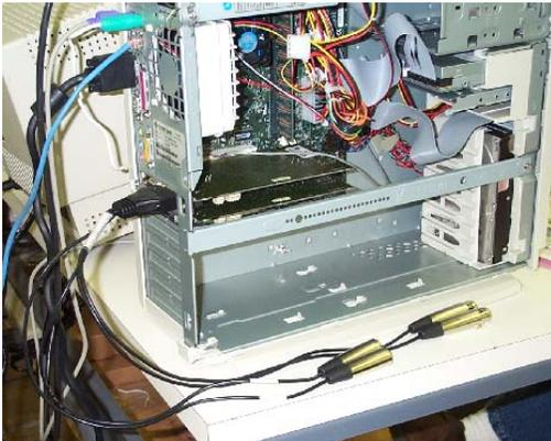
**Access to multiple audio cards is required to record AND play back simultaneously on the same workstation.**
