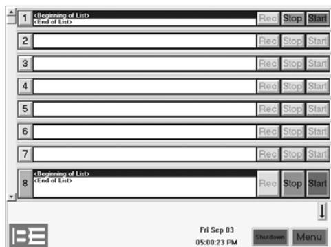
AVNet is basically an automated tape recorder. Using an AudioVAULT playlist, you can program AVNet to start recording an AudioVAULT cut at a specified time.
